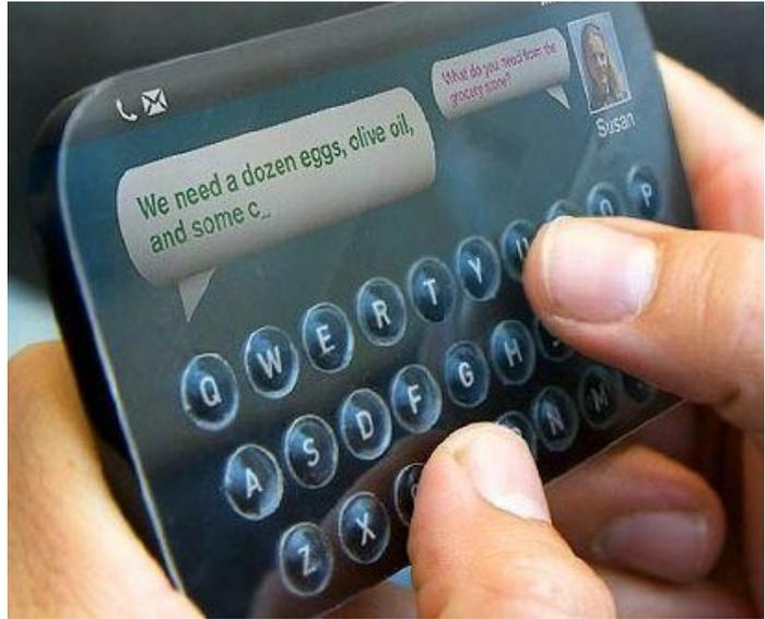
Well, Tactus uses microfluidic technology to create physical buttons that rise from the touchscreen to give users the experience or feeling of operating a physical keyboard. When no longer needed, the buttons recede back into the touchscreen, leaving no trace of their presence.
