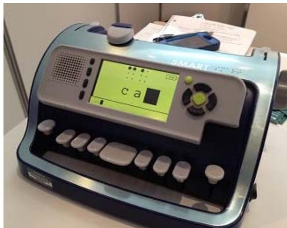
The LED screen displays print in a range of contrasting colours for low vision users, as well as SimBraille or large print! SMART Braille has a USB port for saving work as a .txt file and transfer of files from one device to another, a headphone jack and volume control. The battery is rechargeable and removable. SMART Braille can also work as a mechanical device, without the audio or visual outputs.
